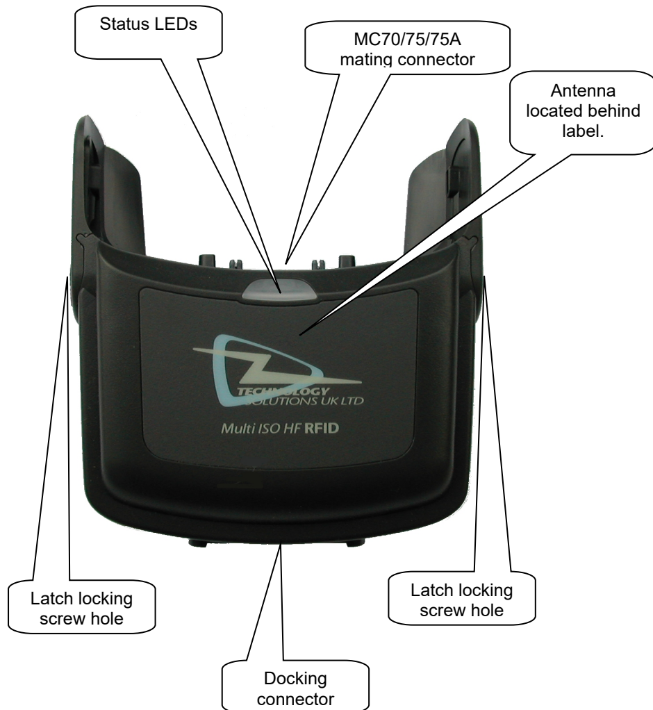
Figure 1: The parts of the RFID 1059
