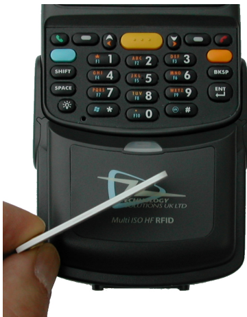
Figure 4: Presenting a transponder to the RFID 1059
